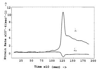
**Figure 2** Strain rate variation versus time with respect to Figure 1. Curve  $\dot{\varepsilon}_r$  corresponds to the data of Figure 1(a), and  $\dot{\varepsilon}_{el}$  corresponds to the data of Figure 1(b).
