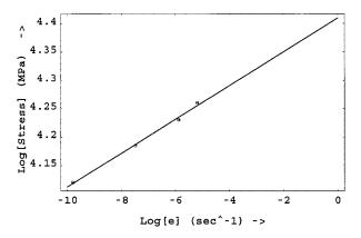
**Figure 8** Yield stress versus strain rate plotted logarithmically at four different strain rates examined.
