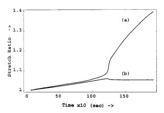
**Figure 1** (a) Strain variation versus time for the zone with maximum deformation and (b) a representative zone that deforms elastically for the crosshead speed of 0.1 mm min.
