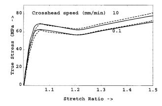
**Figure 9** True tensile stress-strain plots of polycarbonate at two crosshead speeds. Dashed lines represent theoretical results; solid lines represent experimental results.
