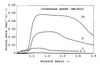
**Figure 4** Strain rate of zone with maximum elongation with respect to the stretch ratio for four different crosshead speeds tested.
