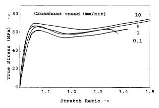
**Figure 7** True tensile stress-strain plots of polycarbonate at four different crosshead speeds with respect to the zone with maximum elongation.
