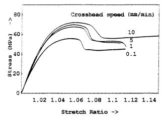
Figure 6 Engineering tensile stress-strain plots of polycarbonate at four different crosshead speeds.
